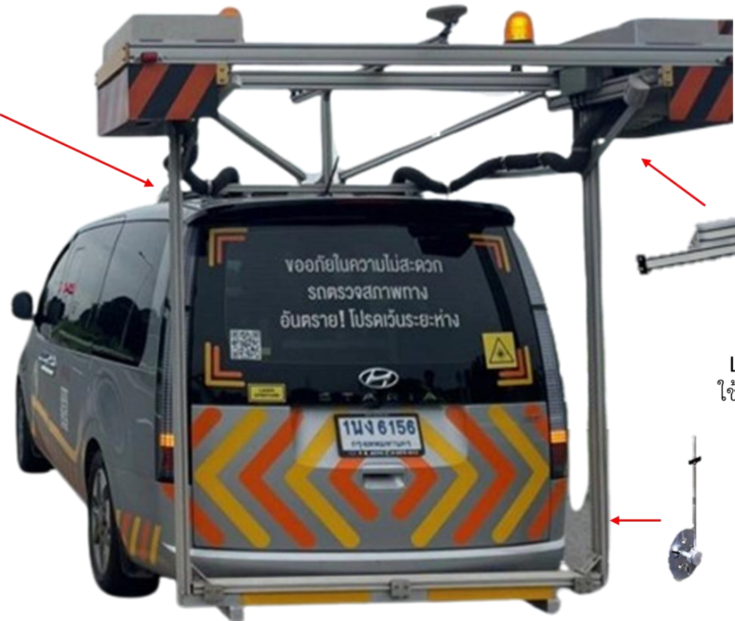
Laser Crack Measurement System (LCMS)
